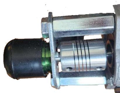
Over time the motor-sensor coupler bolts may get loose and the neutral motor position can get malaligned from normal (often the arm moves just a bit higher than horizontal). If this is the case perform tests (see section 5.4) to make sure motor is moving correctly first or consult DOF Reality support.
